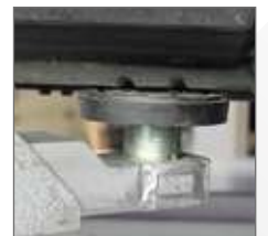
The support disc of the swing arm can be positioned very accurately at the appropriate lifting points under the vehicle.
