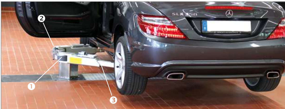
The support disc of the swing arm can be positioned very accurately at the appropriate lifting points under the vehicle.
